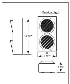
MOUNT 60" ABOVE FLOOR TO BOTTOM EXTERIOR TRAFFIC SIGNAL 6"W X 12"H X 4"D CENTER HOUSING ABOUT 90" ABOVE GRADE FOR TRACTOR TRAILER SERVICE. **EVR 600 VEHICLE RESTRAINT** MOUNT CENTRAL TO DOOR OPENING AGAINST DOCK FACE.
