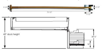
INSTALLATION: Requires mounting of restraint unit, operating bar storage bracket, and when including the Light Communication System, control panel, exterior lights and signs, in strict accordance with McGuire installation instructions. Mechanical installation is recommended to be performed only by authorized McGuire representative.
