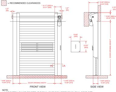
\*INDICATES A RANGE OF SIZES. THE FINAL DIMENSION DEPENDS ON FINAL DOOR SIZE.
