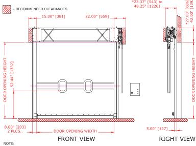
1. INDICATES A RANGE OF SIZES. THE FINAL DIMENSION DEPENDS ON FINAL DOOR SIZE.
