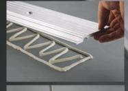
Excaliber<sup>TM</sup> heavy duty aluminum thresholds are made of 6061-T6 aluminum and come in six standard lengths up to 20'4" with either 4" or 6" widths. Sold on its own with pre-drilled counter sink holes, 3/8" anchors and adhesive.
